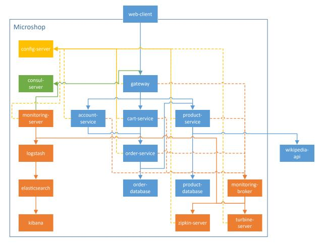
Figure 9.2: Microshop services with its infrastructure. For sake of visibility the registration of all services and servers (including the gateway) to the consul-server, and the aggregation of the logs by the agents to logstash.
