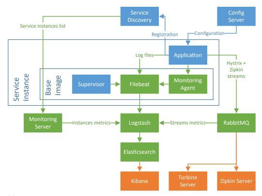
(a) Overview. The monitoring system is in green and some monitoring dashboards are published by the components in orange. Note that the direction of the arrows shows the data flow.
