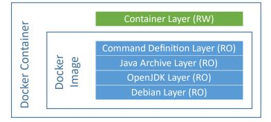
Figure 4.2: A Docker image is composed of many read-only (RO) layers. When this image runs as a Docker container, a thin read-write (RW) container layer is added on top of the image layers.
