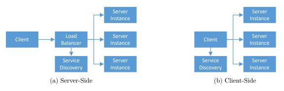
Figure 2.5: Load Balancing
