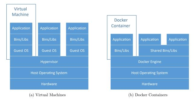
Figure 4.1: Comparison between virtual machines and Docker containers
