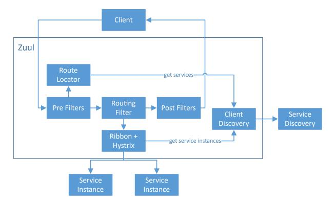
Figure 7.1: Zuul Overview. One interesting pre-filter is PreDecorationFilter which maps the request URL to a service ID using the route locator. The routing filter uses Ribbon to load balance the requests.
