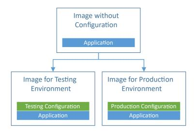
Figure 7.8: In the embedded configuration strategy, we firstly build an image without any configuration. Then, this image can be extended with the configuration of each environment.
