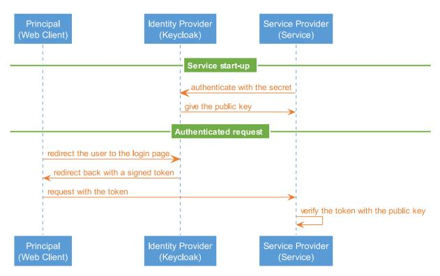
Figure 8.1: Authentication sequence with Keycloak
