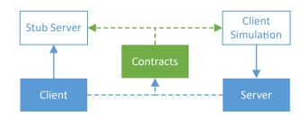
Figure 2.3: In contract testing, the client and the server agree on some contracts and these latter generate a stub server and tests which simulate the client.
