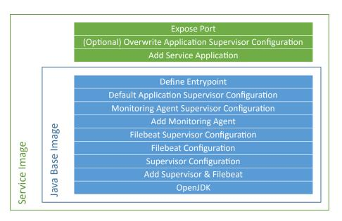
Figure 7.5: Layers of an Image with Supervisor built from listing 7.8
